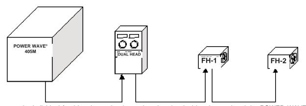
In this case the individual feed heads need to be assigned to the dual head control and the POWER WAVE® 405M auto mapping disabled and the Equipment Groups set on (See Figure A-8). (See the Feeder documentation for information on setting the feeder DIP switches)
